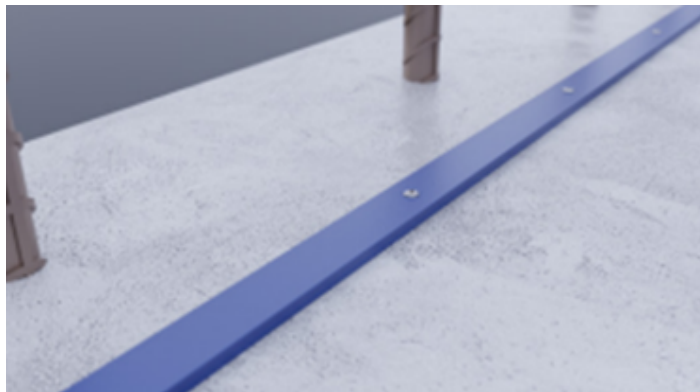
MECHANICALLY ANCHORED BEAD
