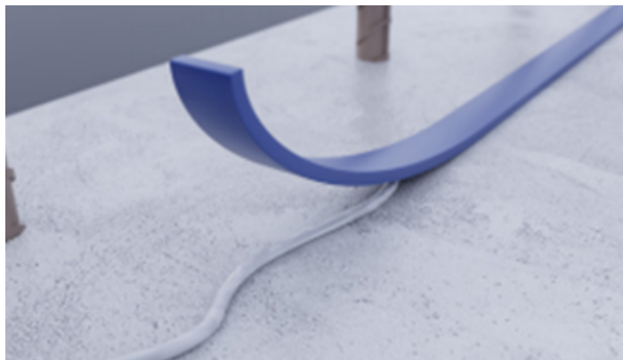
ADHESION THE BEAD WITH PUMALASTIC MS
